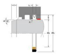
Applications with maximum radial clearance that are using nylon, phenolic, or PTFE bearings must ensure proper clearance in accordance with the bearing recommendations to avoid metal-to-metal contact. Please refer to Hallite Type 87, Type 506, and Type 533 Specification Sheets for this information.
